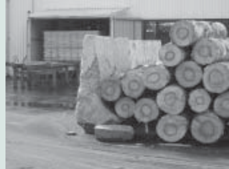
Falling logs are a possible hazard. Logs need to be supported or stacked at a slope of less than 45°
